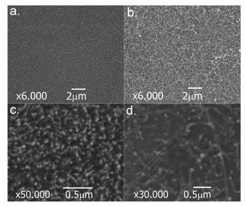
Fig. 1. SEM images under different magnifications of ZnO NWs deposited on Au catalyst/SiO<sub>2</sub> substrate. Left (a and c) correspond to T<sub>S</sub> = 520 °C and right (b and d) to T<sub>S</sub> = 700 °C.
