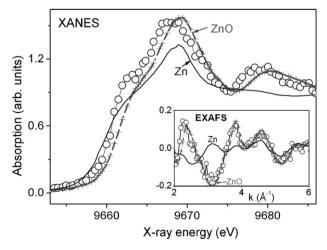
**Fig. 3.** X-ray absorption near the Zn K-edge (XANES) spectrum obtained for a ZnO NW sample deposited at  $T_{\rm S}$  = 700 °C (circles). The reference spectra for a ZnO crystal (crosses and dash-dot line) and metallic Zn (solid line) are also shown for comparison. Inset: Corresponding extended X-ray absorption fine structure (EXAFS) spectrum, together with the corresponding ZnO and Zn reference spectra.
