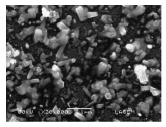
**Fig. 4.** ZnO structures grown on a (100) Si substrate dispersed with Au catalysts under the same deposition conditions as the sample shown in Fig. 1(a and c).
